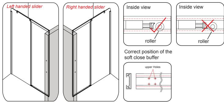
Step.7 Fix the soft closing buffer (no.8) onto the rail as shown above (one for opening and one for closing). There are 4 fixing screw holes in each soft close buffer location inside the rail, make sure to use the upper holes. Also ensure that the soft grey head has been placed in the correct position (please refer to the above di agrams).
